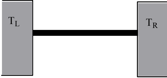
FIG. 1: A schematic representation of a molecular chain connecting two heat reservoirs.
