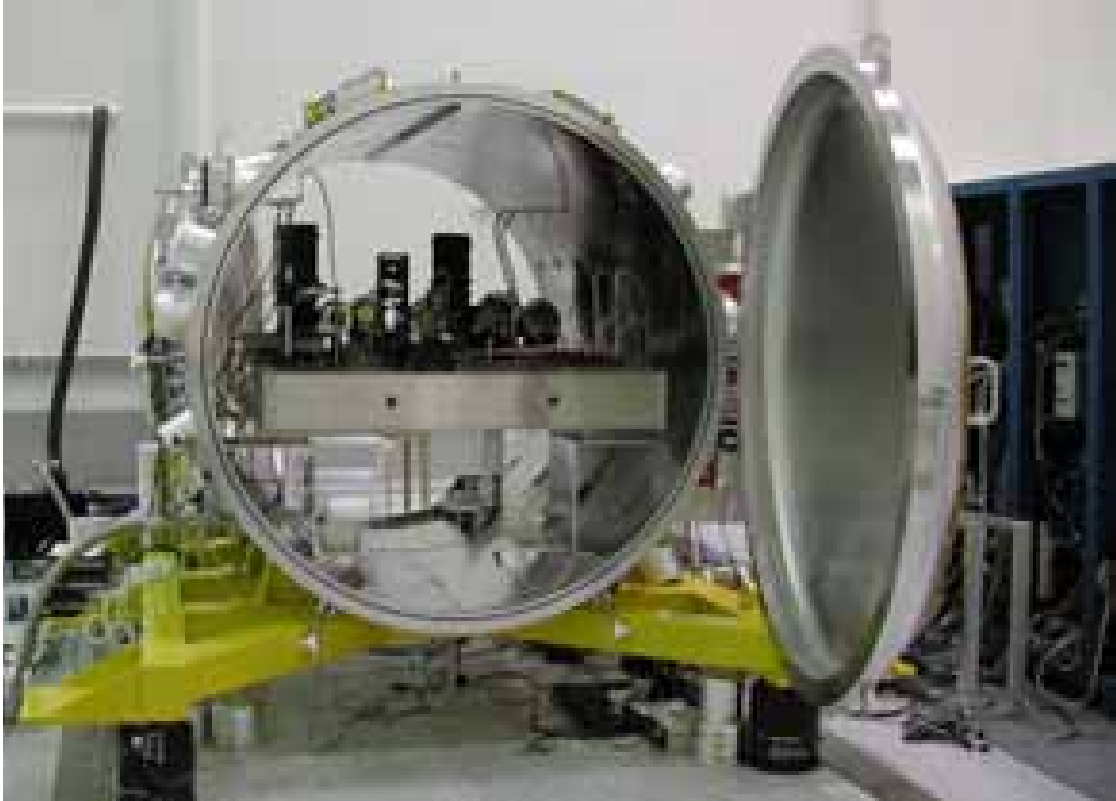
Figure 5: The high contrast imaging testbed is shown within its vacuum chamber at the Jet Propulsion Laboratory in Pasadena, California.
