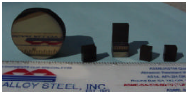
Figure 7. Examples of machined samples from HIPed magnesium diboride. Notice mirror like quality of polished sample on left and third from left. Three small parallelepipeds with sharp corners were machined for high accuracy RUS measurements of elastic constants.
